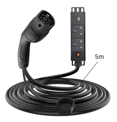
**Waterproof Level:** IP66 **Operating Voltage:** 110-250V **Working Current:** Operating Temperature: -25°C~+55° 15Amp **Maximum Working Power:** 3.75KW Insulator Flammability: UL94 VO Service Life: >10,000Time 2000V Withstand Voltage: Insulation Resistance: >1000MQ Form of Electricity: 1 Phase
